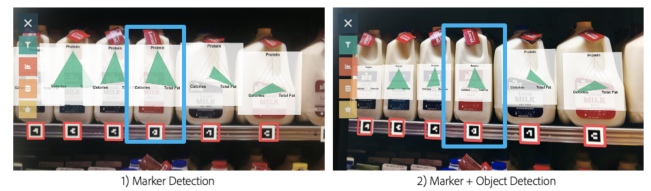
Figure 3: A comparison of product detection and glyph placement results with (a) marker detection only and (b) marker+object detection.
