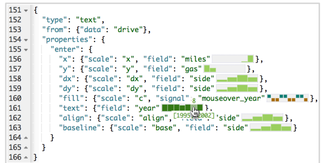
Figure 1. Code augmentations visualize the runtime state of program variables in a Vega [32] specification. A histogram shows the distribution of variables containing set data. Interacting with the year histogram filters all other histograms to only show the data values where the year is between 1995 and 2002 (hand cursor shown here for clarity; in a real implementation the cursor is hidden mid-interaction to aid chart reading). For mouseover_year , a tick visualization depicts value changes.
