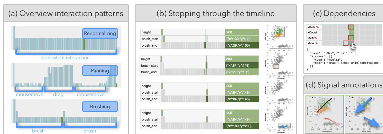
Figure 6.2: The overview, timeline, and signal annotations after performing interactions on a Vega visualization. (a) The overview provides insight into different interaction patterns. (b) Stepping within a pulse allows users to see intermediate states of an interaction. For example, the second scatterplot shows a brush representing the new brush_start and old brush_end . (c) Dependencies are shown as red outlines in the timeline on hover. (d) Signal annotations overlay the visualization, with fill color encoding temporality: from darkest (past), through red (current), to lightest (future).
