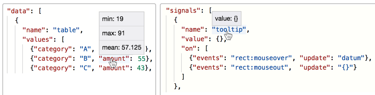
Figure E.2: We augmented the online Vega editor to display a tooltip showing the signal value or summary information about the values of a data field (e.g., the min, max, and mean). The tooltip reflects the general behavior found in existing debugging environments [9]. Note: only the figure was included in the original evaluation materials; this caption was added to explain the content.
